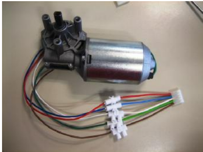
Picture 4: Wire connector joined to the motor wire.
