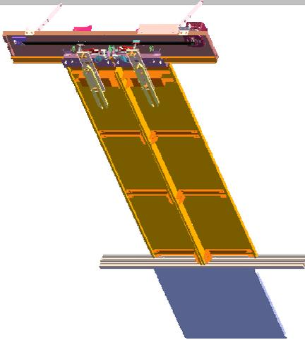
**Principle:** Single rail door drive, 2 panel, central opening. VVVF control. Can be used with the existing door panels or new panels.
