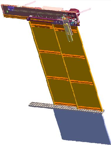
**Principle:** Single rail door drive, 2 panel, telescopic. VVVFcontrol .
